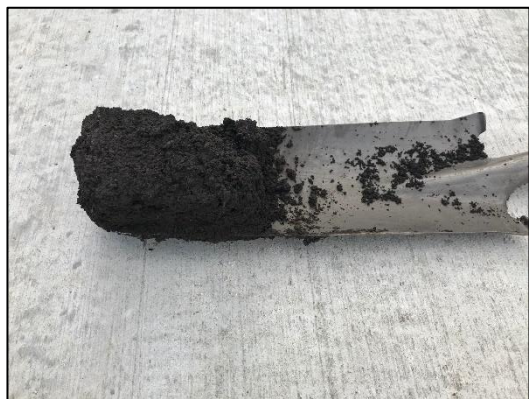
Soil slice for soil aggregate stability taken with tilling spade, trimmed down to 1-inch thick slice. Soil sample depth is 0-6 inch.
