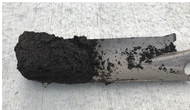
Figure 3. Soil slice for soil aggregate stability taken with tiling spade. Soil sample depth is 0-6 inch.
