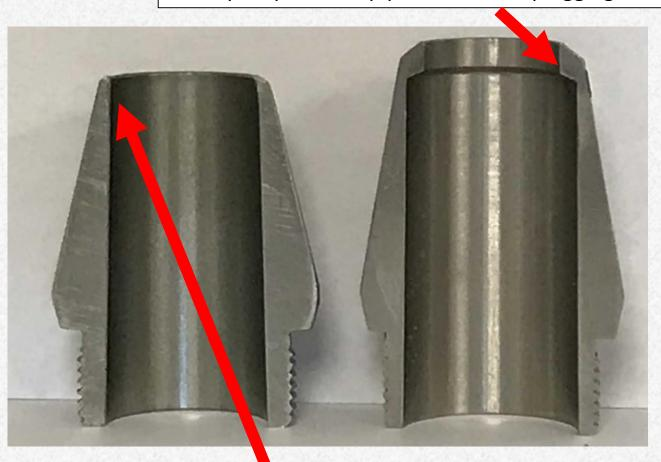
Dry Tip - Sharp cutting edge and slow taper prevent soil core from falling out in dry conditions
