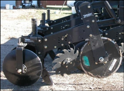
Fertilizer (10-34-0) placement methods: Deep band (during strip tilling)
