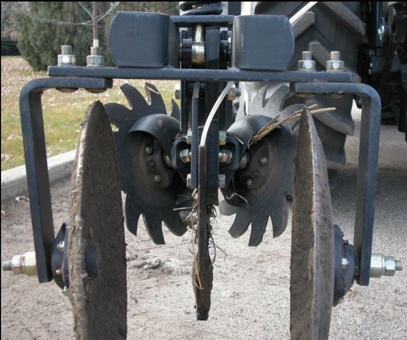
Fertilizer (10-34-0) placement methods: Deep band (during strip tilling)
