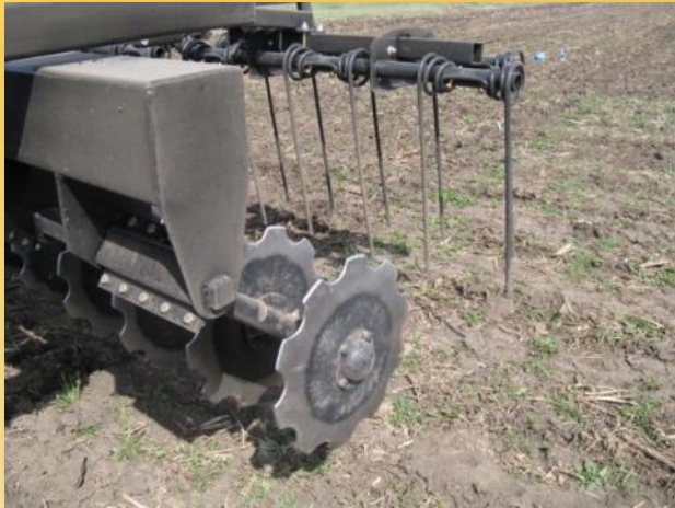
Gates Magnum Coulter at 0 and 7.5 degree pitch
