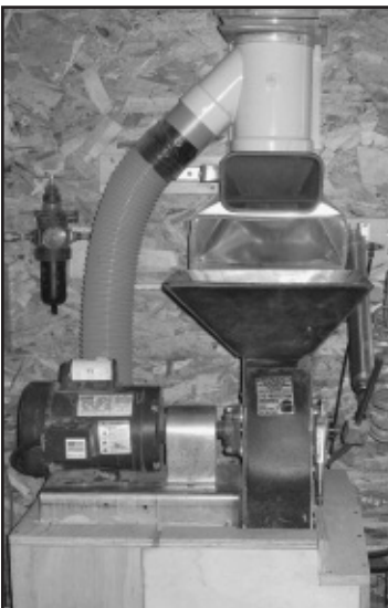
New grinder dust control.
