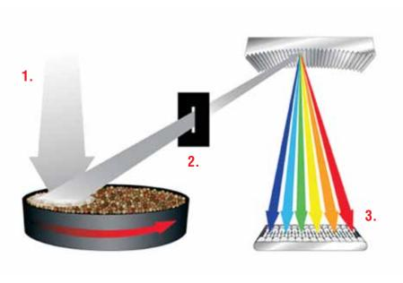
The principle behind NIR is specific organic molecules absorb specific wavelengths of near infrared light energy. The absorptions are directly correlated with the concentration of the organic molecules in the sample. This relationship must be correlated with a primary technique, otherwise known as wet or bench chemistry. Therefore, the NIR is dependant upon the wet chemistry methods to attain the linear relationship between the molecular absorptions and the actual constituent concentrations.
