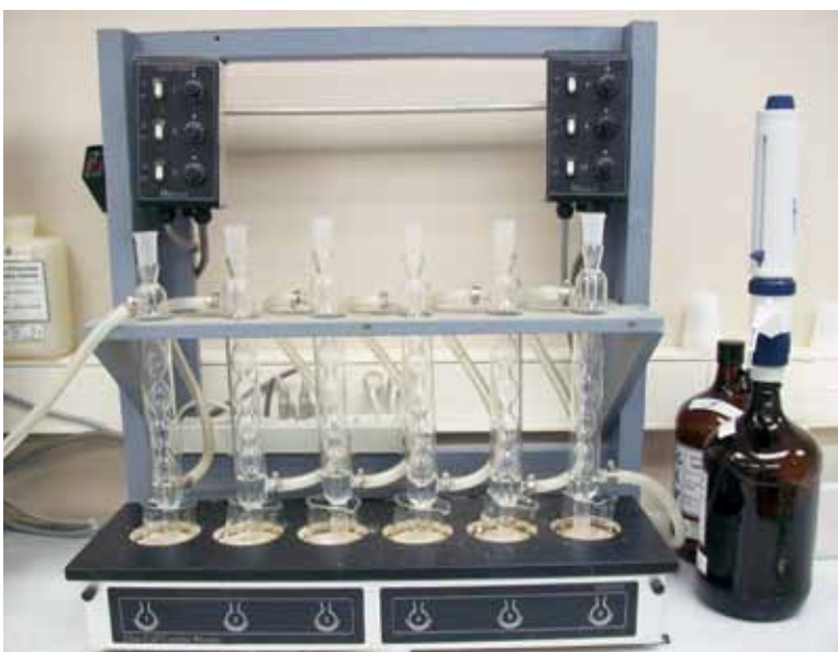
Condensing towers used to analyze microbial biomass
