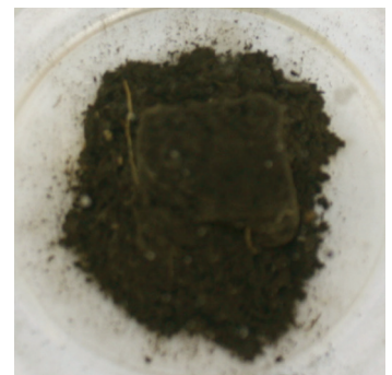
Sodic Soil - 1 hour 45% Sodium - Dispersion Continues
