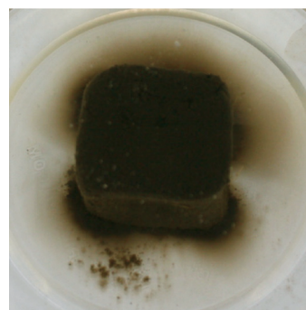
Sodic Soil - 2 minutes 45% Sodium - Dispersion Starting
